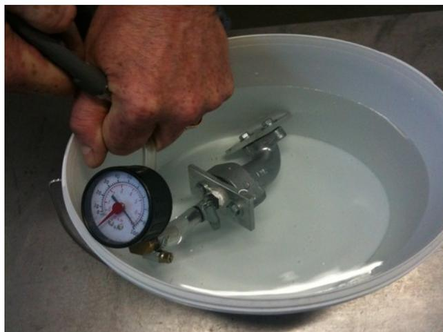
Impregnated part pressure tested up to 10 bar and 200 °C
