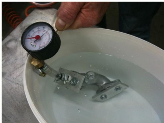
Failed pressure test - Air bubbles
