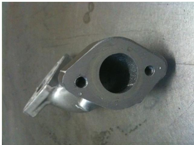
Intake manifold of a light motorbike
