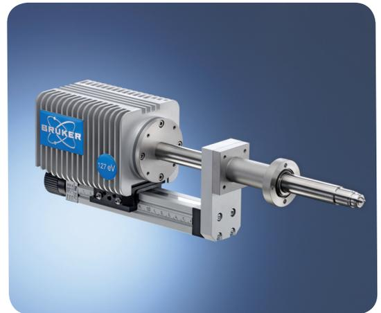
Thanks to its optimized electron trap, interference-free analysis is guaranteed even at low excitation energies.
