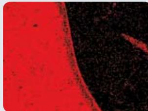
Re-indexing shows that Taenite (fcc) was misindexed as Kamacite, the missing phase is a carbide (Cohenite)
