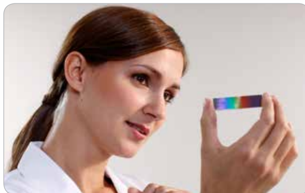
A linear variable long pass filter slide (shown) is one of many specialized components that make up the CLARIOstar's sophisticated LVF Monochromator system.
