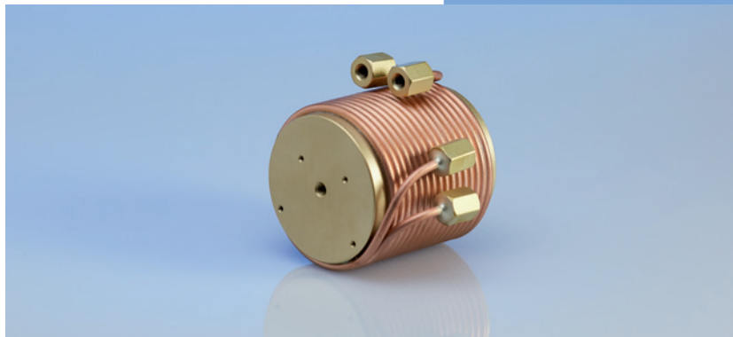
DualChannelTCD with integrated heat exchanger for identical temperature of reference and analysis gases
