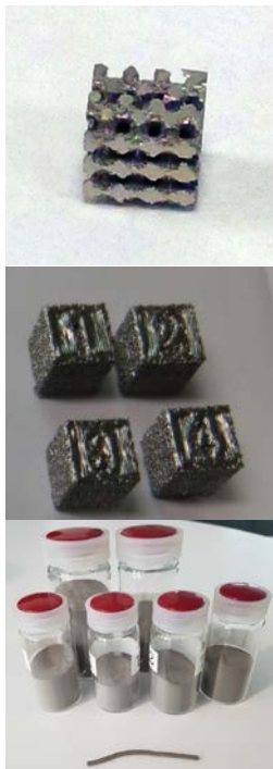
Figure 1. Example of different SLM produced test specimens (cubes) and the initial powder metal used.
