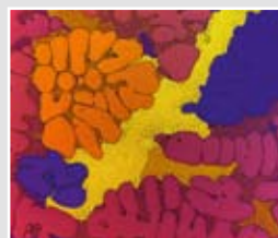
AlNi 3.5 anodized according to Barker Polarization contrast EC Epiplan-NEOFLUAR 20x/0.50
