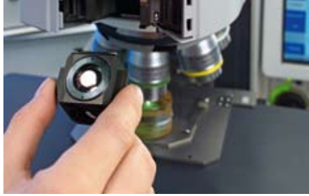
More options, faster handling: the reflector turrets with Push&Click modules
