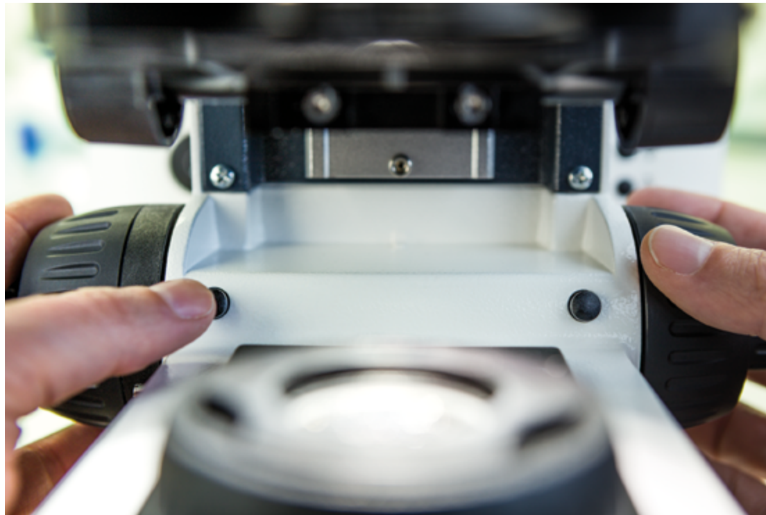
Axioscope 5: Snap button for image acquisition on both sides Axioscope 7: Snap button (right) and stage control button (left)
