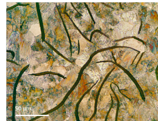
Flake graphite in cast iron, etched sample Images provided by University of Applied Sciences, Aalen, Germany
