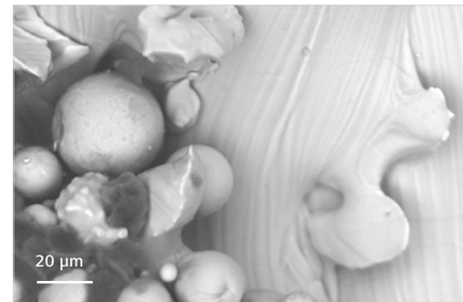
Surface of additively manufactured titanium alloy component. Sample provided by TWI Ltd
