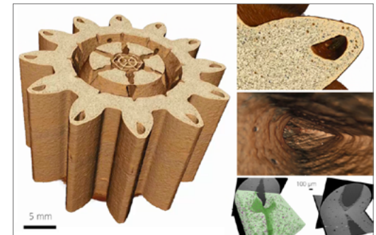
3D scan of Al component produced by additive manufacturing and, inset, internal porosity imaged via X-ray microscopy
