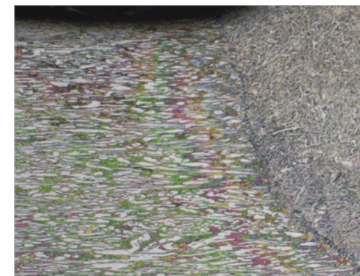
Parent to weld interface in duplex stainless steel. Sample provided by TWI Ltd
