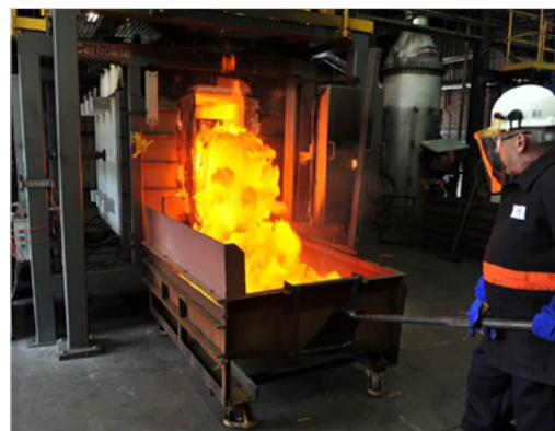
Pushing the 350 Kg Pilot Coke Oven at the Materials Processing Institute, Middlesbrough, UK. Photograph provided by the Materials Processing Institute, UK.
