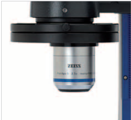
Objective PlanApo S 3.5x mono on Objective slider S/doc ■ For axial mode only ■ Free working distance FWD= 16 mm ■ Max. possible resolution of 1,510 LP/mm (equals 0.3 µm)
