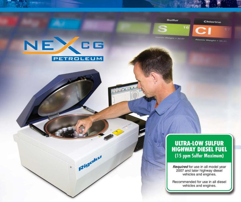
Rigaku NEX CG is a Cartesian geometry energy dispersive X-ray fluorescence (EDXRF) analyzer that delivers rapid qualitative and quantitative determination of major and minor atomic elements in a wide variety of sample types of interest to the petroleum industry.
