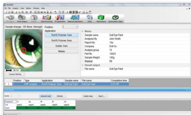
Point Analysis interface, available in a variety of languages, is used for small spot measurements. A live camera display is shown in the left window.
