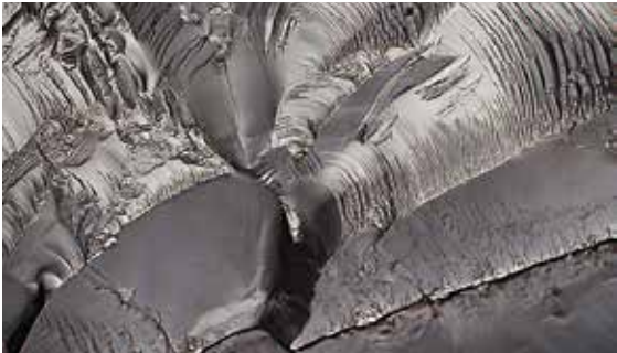
Fracture of silicon
