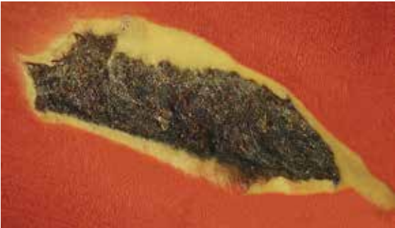
Paint peeling surface (350x)
