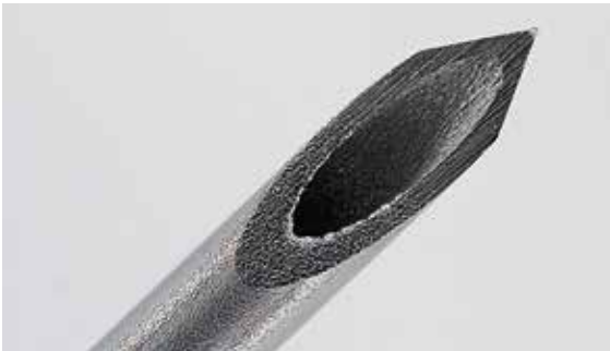
Medical injection needle (140x)
