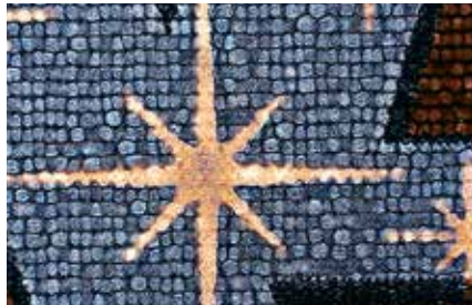
Printed surface of package (35x)
