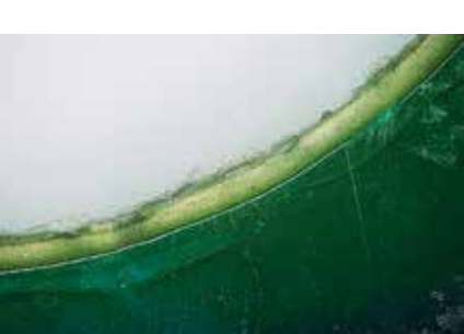
Scratches on circuit board (80x)
