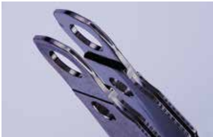
Swing arm in HDD (80x)
