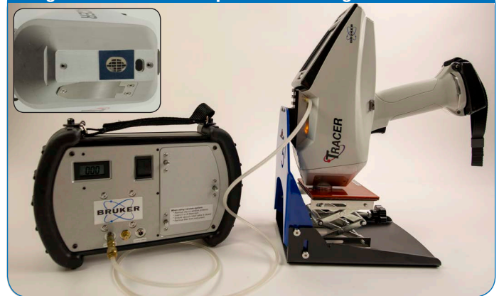
Figure 3: Vacuum setup & TRACER 5i gridded window
