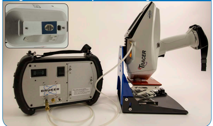
Figure 3: Vacuum setup & TRACER 5i gridded window
